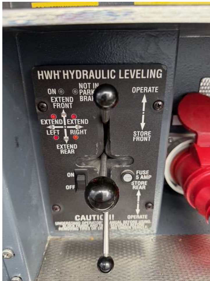
2 front and 2 rear cylinders
